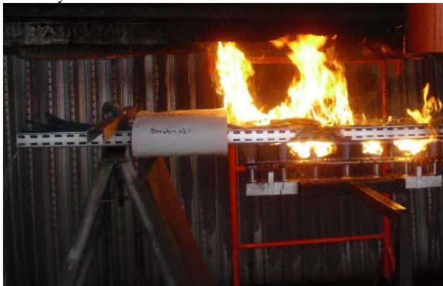
Figure 5.4.5.1 Configuration of cable trays with fire screen.
